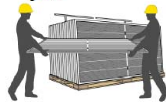
3) Place the stand supporter that is higher or wider than the module in order to avoid hitting and damaging the glass.
