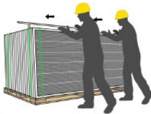
4) Cut off all the horizontal packing belts; when there are 1 or 2 vertical packing belts remaining, push the module gently to tilt toward the stand supporter.
